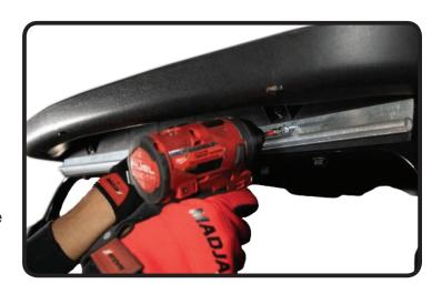
Identify the driver side track pc. (B). Align the three notches in the metal track to the ribbing in the top. Using a measuring tape and marker, if necessary, mark two holes where you will drill into the top to secure the driver side track. Using a 3/16" drill bit drill into the top in the respected hole locations. Using the supplied nut, bolt, and washer, secure the track to the top using a 10mm socket and flat head screw driver.
