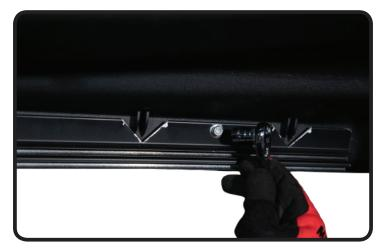
Identify the rear track pc. (C). Using a measuring tape and marker, if necessary, to mark 2 holes where you will screw track to the rear struts of the cart using self tapping screws.
