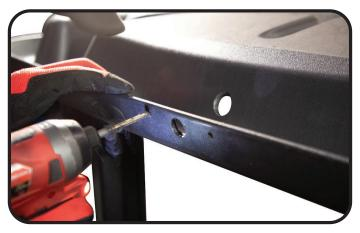
Feed the wire through the new hole and secure the camera to the top using a 4mm allen and 8mm socket.
