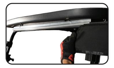
Work your way around the vehicle and zip up the enclosure to ensure proper fitment.
