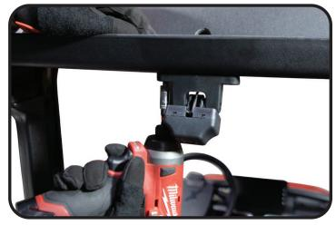
Using a flat head screwdriver pop the tab open on the track holding the camera wire in place. Disconnect the camera wiring and remove the camera from its current location.
