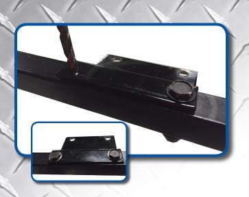
Using a 5/16" bit, drill through strut using front bracket as a guide as shown. Use 8mm x 40mm bolts and 8mm Nylock nuts and tighten.
