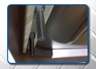
Connect the strut brackets to the top extrusion using 8mm carriage bolts, hand tighten hardware first. Once all bolts are in place then tighten.
