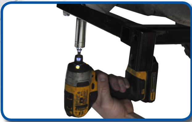
Using a 17mm socket tighten hardware. Be sure the U-bolt is tightened evenly as shown.
