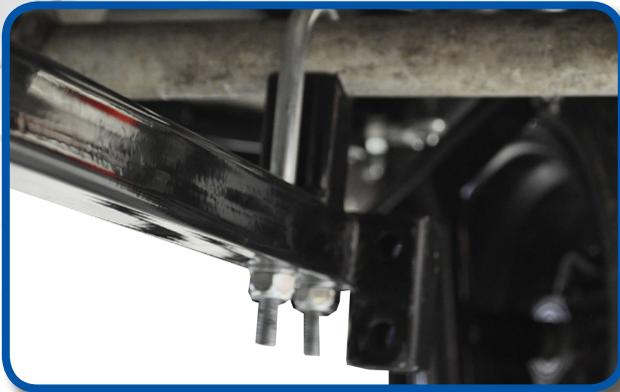
Tighten all U-Bolt hardware with 17mm socket.\*Be sure to tighten all U-bolts evenly.
