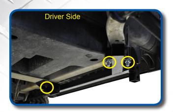
Now that all mounting hardware is in place, tighten all hardware, be sure that U-bolt is tightened evenly as shown.
