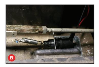
C) Plug the 2 bullet connectors from the brake switch into the corresponding bullet connectors on the light kit harness. Secure all wiring so that it is away from moving parts.
