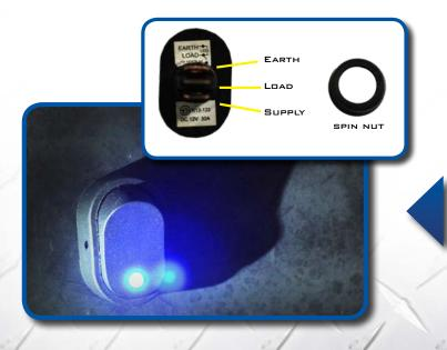
Using a 15/32" drill bit, find a desired location on your golf cart dashboard to mount your rocker switch for hazard lights. Ensure your location is free of obstacles and will not affect dash reattachment.
