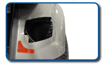
Remove factory tail light hardware. Retain hardware.
