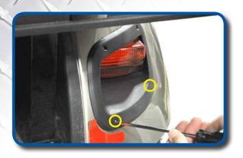
Install new tail lights using retained hardware.
