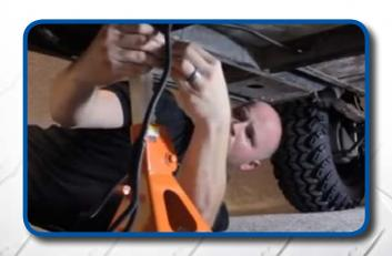
Lift the cart and place jack stands to support. Feed the headlight portion of the harness down through the front of the battery comparment. Route the wiring harness through the holes under the frame. Run long tail light wire under the seat and over the rear tire well on the passenger's side. Run short tail light wire under the seat and over the rear tire well on the driver's side. Loosely secure with wire ties until all lights have been installed.
