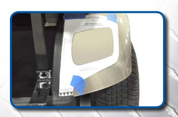
Feed the tail light harness through the back of the cart. Attach rear tail light wire harness as shown. Secure wire with ties.
