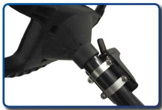
Attach turn signal back cover to turn signal assembly.
