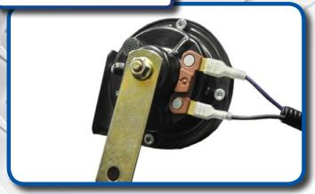
Attach horn to purple and black female spade connectors and secure horn to metal framing under the front cowl using supplied hardware.
