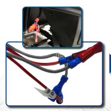
At the headlight, unplug the connectors in the Grey and Red/White wires.
