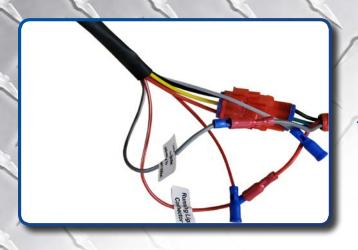
Plug the Grey and Red/White wires from the harness into the corresponding connectors on the headlight.
