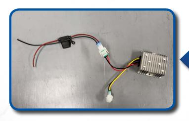
The voltage converter included must be used on 36 volt & 48 volt electric carts. Connect the red wire with the fuse to the positive terminal of the battery pack. Connect the black wire to the negative terminal of the battery pack.
