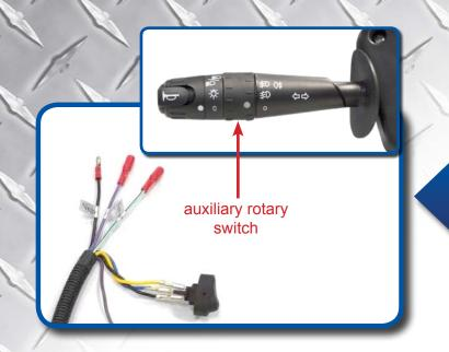
The turn signal handle has a secondary, 2-position rotary switch for auxiliary 12 volt lighting, There is one common negative wire and two positive wires to run two different sets of auxhillary lighting. Additional wiring and lighting not included.
