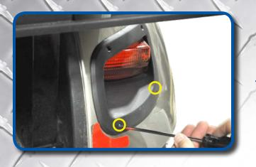
Install new tail lights using retained hardware.
