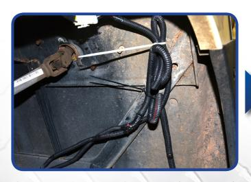
Secure remaining harness under cowl using provided ties.
