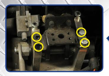
Loosen all 4 bolts holding the brake pedal stop bracket to the brake assembly.
