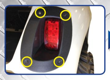
Place tail light into the rear of the vehicle. Insert four screws into Tail light using supplied hardware.
