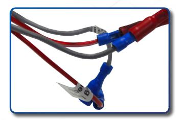
At the headlight, unplug the connectors in the Grey and Red/White wires.
