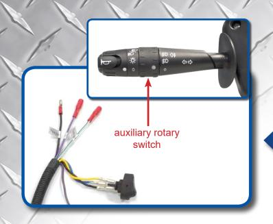
The turn signal handle has a secondary, 2-position rotary switch for auxiliary 12 volt lighting, There is one common negative wire and two positive wires to run two different sets of auxhillary lighting. Additional wiring and lighting not included.
