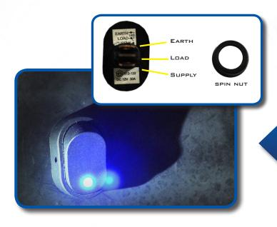
Using a 15/32" drill bit, find a desired location on your golf cart dashboard to mount your rocker switch for hazard lights. Ensure your location is free of obstacles and will not affect dash reattachment.
