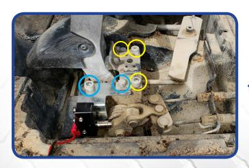
Using a 10mm socket and a 6mm Allen wrench, remove the two bolts circled in blue and loosen the three bolts circled in yellow. Slide the brake switch bracket between the pedal stop and the pedal group bracket. Reinstall the two bolts circled in blue. Adjust the switch so it is accuated after the pedal begins to move. Tighten all bolts.
