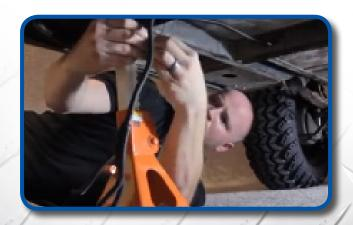
Lift the cart and place jack stands to support. Feed the headlight portion of the harness down through the front of the battery comparment. Route the wiring harness through the holes under the frame. Run long tail light wire under the seat and over the rear tire well on the passenger's side. Run short tail light wire under the seat and over the rear tire well on the driver's side. Loosely secure with wire ties until all lights have been installed.
