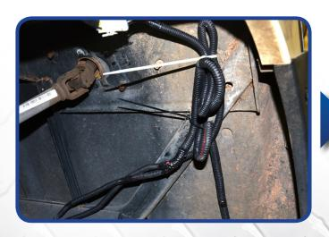
Secure remaining harness under cowl using provided ties.
