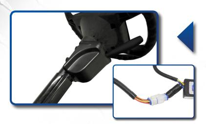
Attach turn signal back cover to turn signal assembly.
