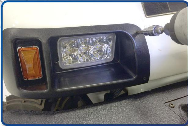
Place headlight into the front of the vehicle. Insert four screws into headlight using supplied hardware.
