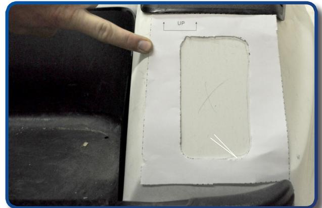
Drill a pilot hole and cut out the shape of the tail light.
