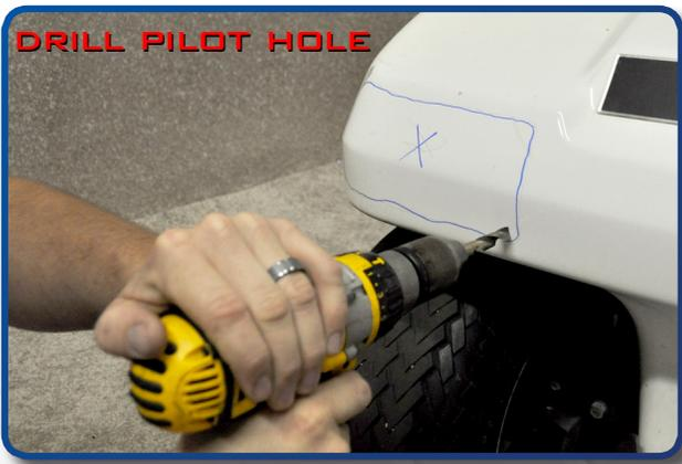
Draw the inside of the template out with a writing utensil. Next drill a pilot hole so you will have a starting point to begin cutting.
