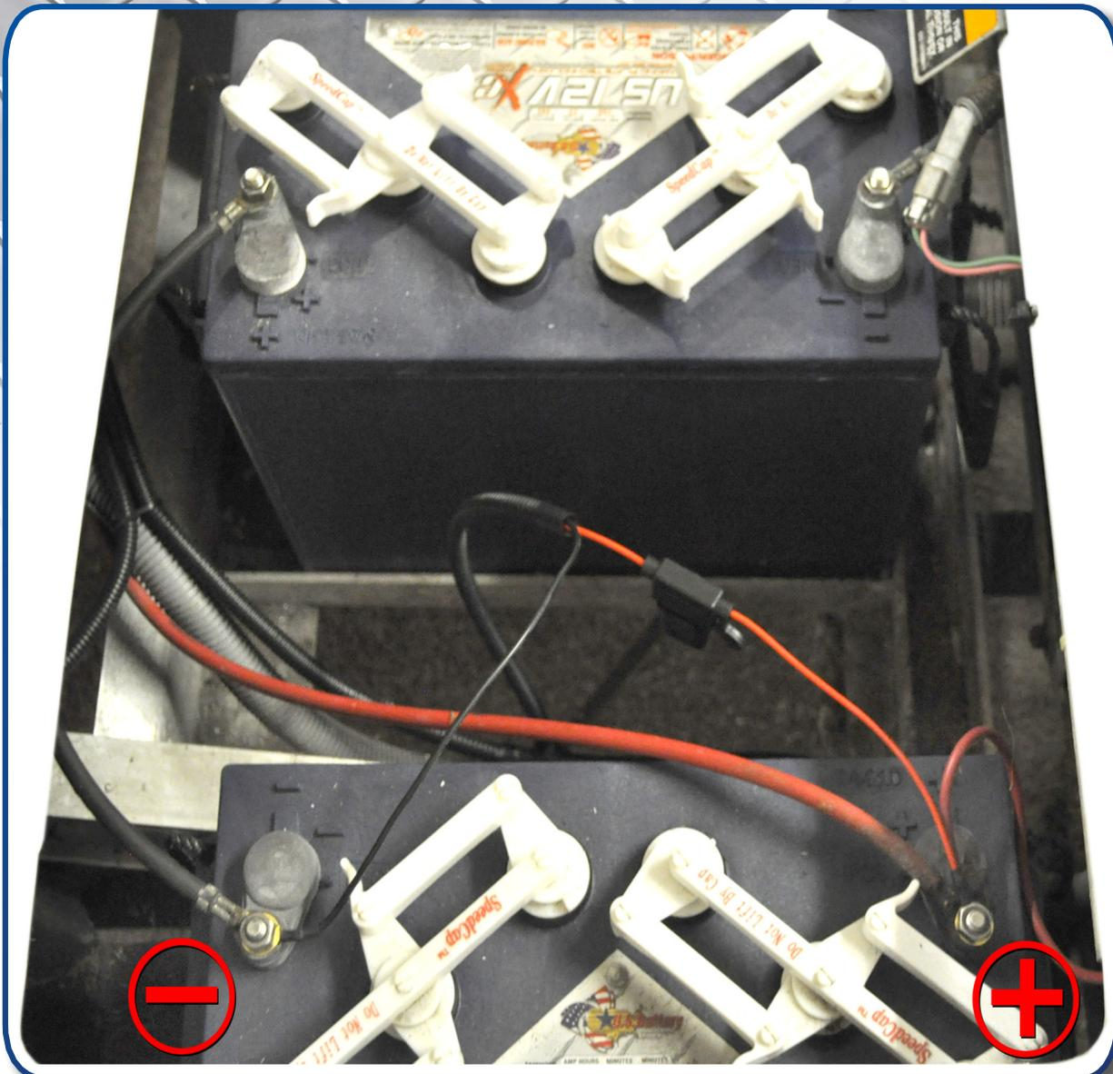
If you have 12 volt batteries wire the harness to the battery as shown. If you have 8 Volt batteries a Madjax 16/12 voltage reducer will be necessary.
