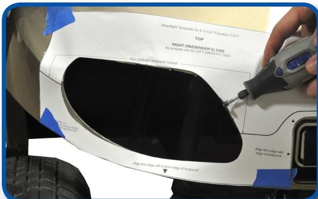
Cut out the shape of the headlight. Use the cutting tool to remove the excess trim. \*Flip template over repeat process on the other side.
