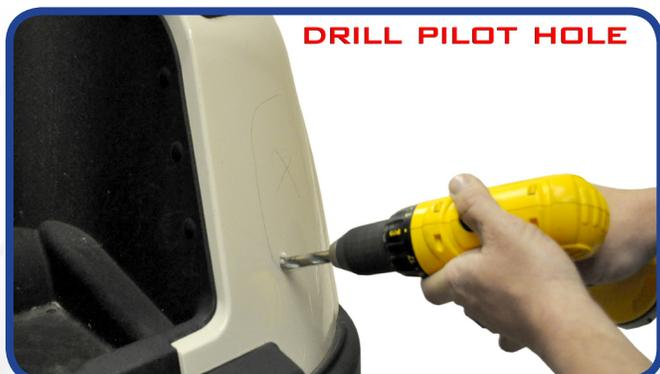
Draw the inside of the template out with a marking pen. Next drill a pilot hole so you will have a starting point to begin cutting.
