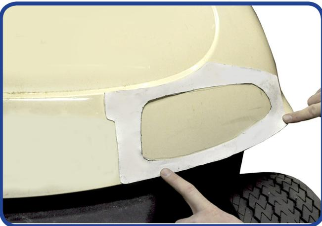
Drill a pilot hole and cut out the shape of the headlight.
